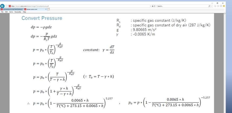
Reference) World Meteorological Organization / CIMO/ET-Stand-1/Doc. 10 (20.XI.2012) <u>https://www.wmo.int/pages/prog/www/IMOP/meetings/SI/ET-Stand-1/Doc-10\_Pressure-red.pdf</u> (p6 eq(4)) Keisan 2018/1/24 Here is the derivation of the equation used to determine the Mean Sea Level (MSL) Pressure, if you are keen to see how it was derived, but we will just use the formula for this exercise.
