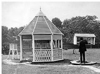
Figure 13: Stevenson Screen on left, thermometer house in middle and Glaisher Screen on right, Adelaide Observatory circa 1900.- BOM
