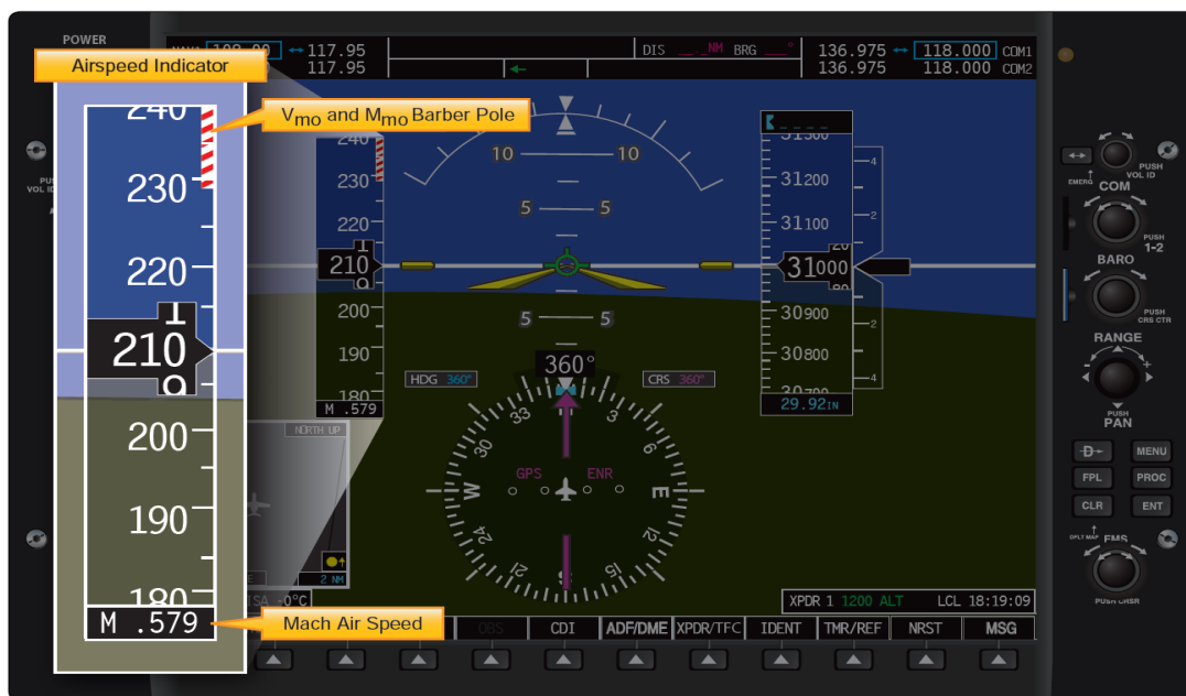
Figure 4: Jet Electronic AirSpeed Indicator Source: FAA Note the use of a strip to show trends as well as the digital output. For more explanation please click on link provided
