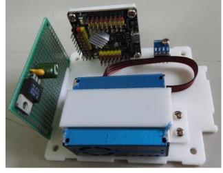
again selected so that the M3 screws could be screwed directly into the plastic.
