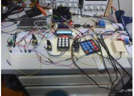
While the breadboard (as it is called) proved that the system worked, it was hardly usable in real life.
