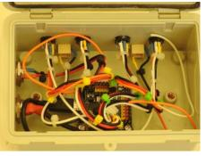
Once the prototype Arduino was completed, it was time to make the a sensor prototype or two. The first is a set of ground thermometers. There sensors are set to measure the temperature at ground level, 10cm, 20cm deep, 50 cm deep and 100 cm deep. As you can see from the photo below, the construction is very simple. The temperature sensors are spaced out and taped in place. They are then put into a piece of irrigation pipe so it can be sunk into the ground to the correct depth easily.
