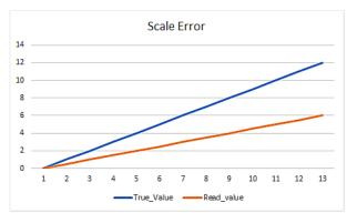
As you can see from a graph of a scale error, it looks quite different from the offset error as the readings meet at zero (0) and diverge the further away from zero that the true value gets.
