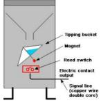
One sensor where this is not so easy is with the tipping bucket (or tipping spoon) rain gauge. As shown by the diagram to the left, the tipping bucket/spoon rain gauge works by a container filling and tipping over to empty. As it tips, a magnet passes a reed switch which sends a pulse to the computer.
